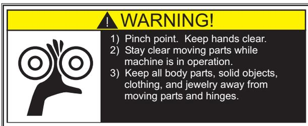
Pinch Label: (2) located on front upright pipes and (1) located on rear angles pipe
