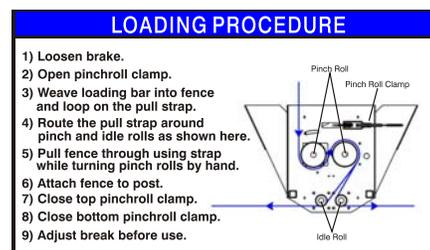
Loading Procedure Label: (1) located on frame and (2) located on front of brake hood
